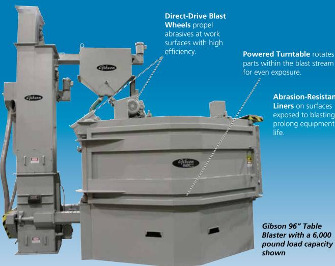
**Abrasion-Resistant Liners** on surfaces exposed to blasting prolong equipment
