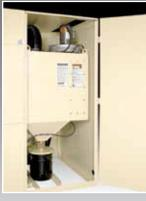
ProFormer<sup>™</sup> cabinets are equipped with cartridge dust collectors to facilitate a quick change of filtration surfaces. These two cartridges have a filtration area of 103 square feet each, providing a total of 206 square feet, and can be replaced in minutes through the cabinet door. As a result, loose dust falls into the cabinet rather than onto the work floor.
