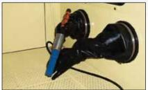
High-intensity lighting, a venturi blast nozzle with lightweight blast hose, and abrasionresistant operator gloves boost productivity.
