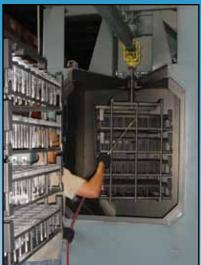
**Pneumatic Trolley** transports heavy loads of parts in and out of the blast enclosure.
