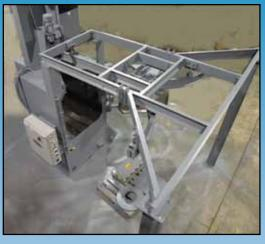
**Y-track** branches into two rails so one fixture can be loaded and unloaded while parts on the second fixture undergo blasting.
